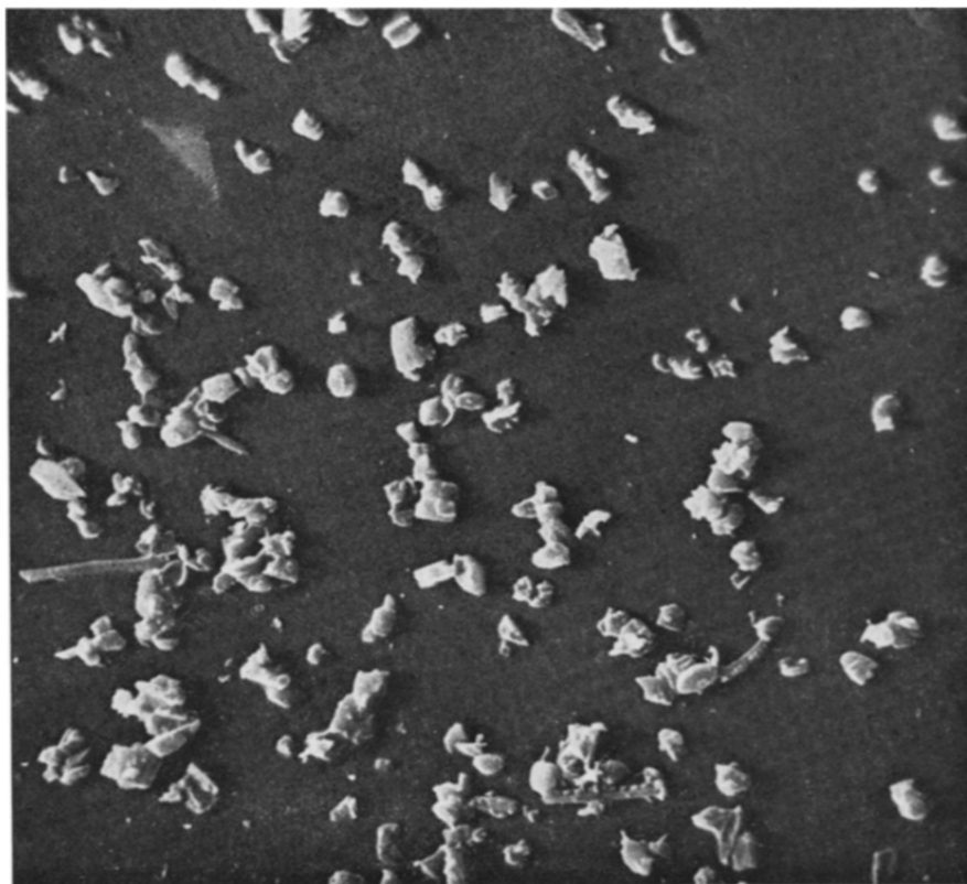
Fig. 3. Scanning electron microscope photograph of a SCOT column coated with Hyflo Super Cel and SE-30. Magnification: 500×.
